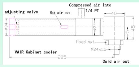
Cabinet Cooler Specifications - M style Stainless Steel Cabinet Cooler only +hose kits:
